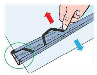
3 Insert the remaining wire thanks to a back forth UP and DOWN movement.
